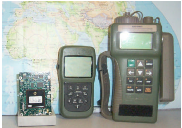
Current military GPS receivers are (from left) the embeddable GPS receiver GB-GRAM, the handheld DAGR and handheld PLGR. See page 2 for more product information.
