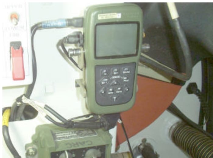
A typical DAGR installation is shown in the Stryker vehicle where the DAGR is connected to external power and antenna; The PC cable is used to provide GPS data to other Stryker mission equipment. In this case, the DAGR can be removed quickly and used by the crew for Situational Awareness if they evacuate the vehicle.
